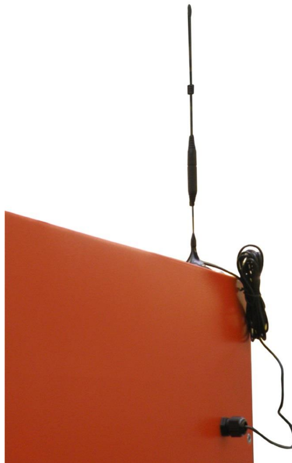
Figure 4.19 GSM antenna positioned on top of the inverter
